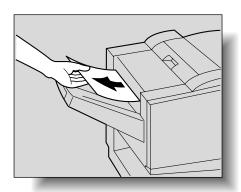
**9** Open the feed guide for the finisher, and then remove any misfed paper.
